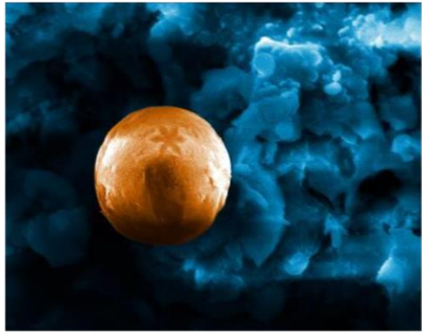
“Rising nano-star”: Scanning Electron Microscopy image of Ti surface (blue), treated by the hydroxyapatite granules (orange) using gas detonation technique (false-colored).
