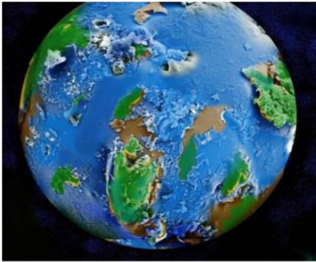
“There’s plenty of room at the bottom: Earth”: Scanning Electron Microscopy image of SiO 2 particle synthesized through the hydrothermal method (false-colored).
